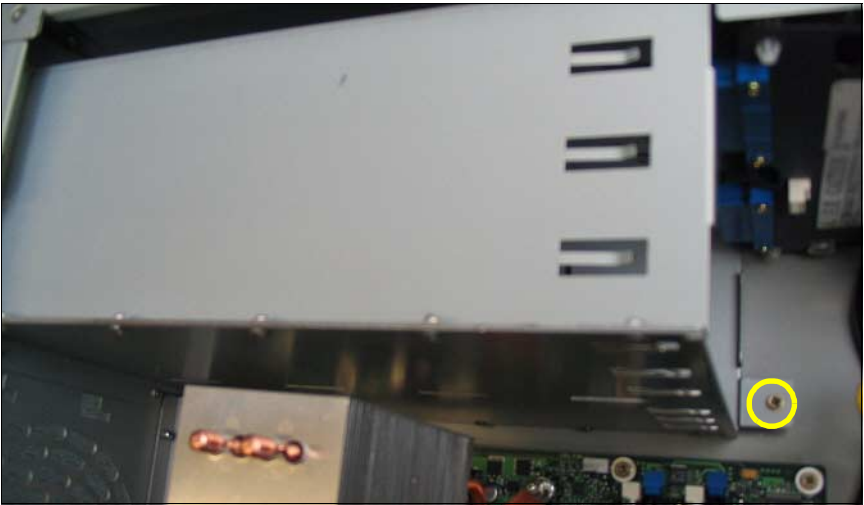
Figure 33: Fastening the PS cage in the housing
